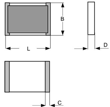
L = Länge, B = Breite, D = Dicke, C = Breite Umkontakt (in mm)
